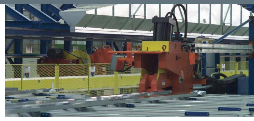
The Granco Clark Controlled Vertical Crush Stretcher delivers maximum gripping control with minimum distortion.
